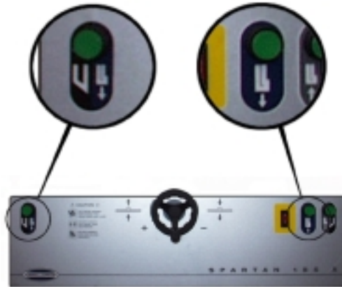
Figure 12 – Clamp Only Buttons
