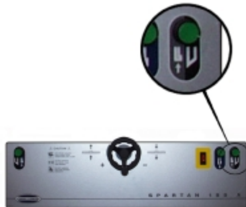
Figure 13 – Clamp Up Button
